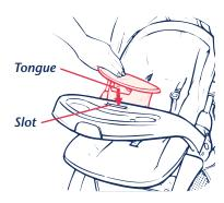
UNLOCKING SWIVELS FOR SMOOTH SURFACES: (swiveling wheels)
